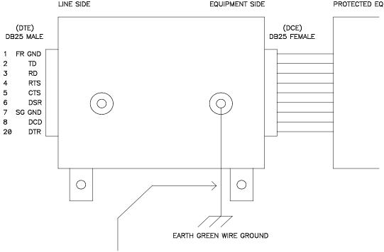
10 GAUGE COPPER WIRE AT 3 FEET LONG. OR BRAIDED CABLE MADE SPECIFICALLY FOR GROUNDING PURPOSES.
